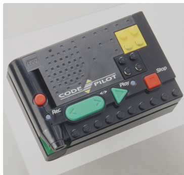
The barcode reader developed for 8479 Barcode Multi-set allowed the set's dump-truck vehicle to be programmed using a sheet of printed barcodes.
