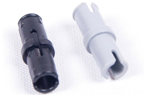
Friction snaps ( left ) are distinguished from smooth snaps ( right ) by the ridges along their length. These ridges resist turning when the snap is fitted into a hole.
