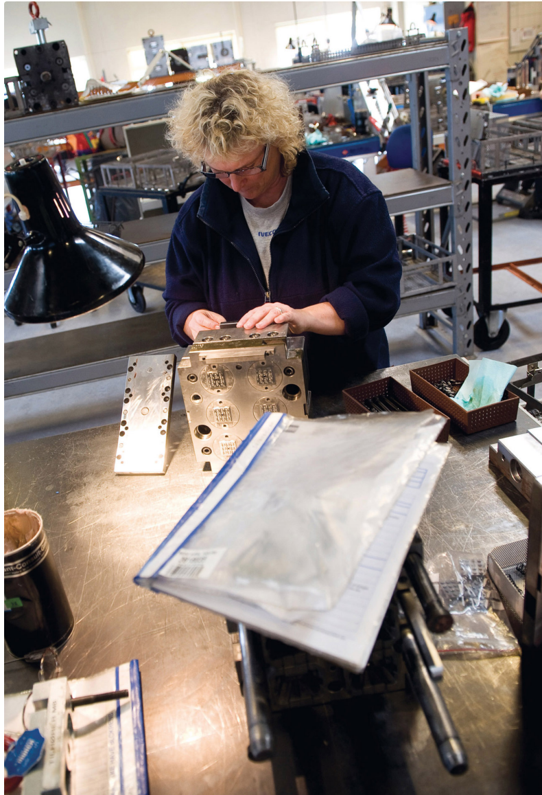
A special division in the LEGO Group factory in Billund, Denmark, regularly maintains moulds.
