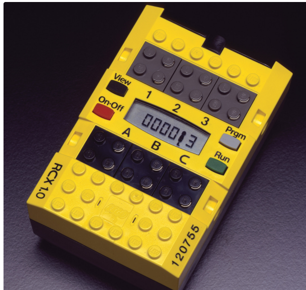
The initial RCX component that was at the heart of LEGO MINDSTORMS.
